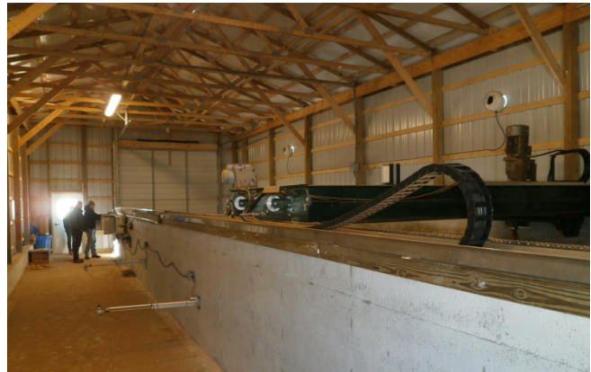
Figure 2. Green Mountain Technology's composting system at Glamour View Farm is housed within a permanent structure. Figure 2. The Earth Flow composting system features automated mixing and aeration equipment. Photo credits: David Kann.
