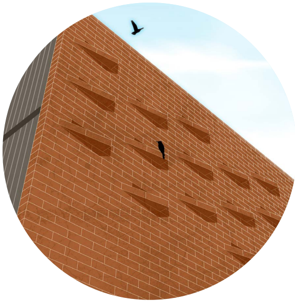
Two views of a high, horizontal band of bird boxes for nesting birds: the boxes are distributed in a running bond pattern that echoes the existing brick bond of the facade. Renderings: Emily Kelly.
