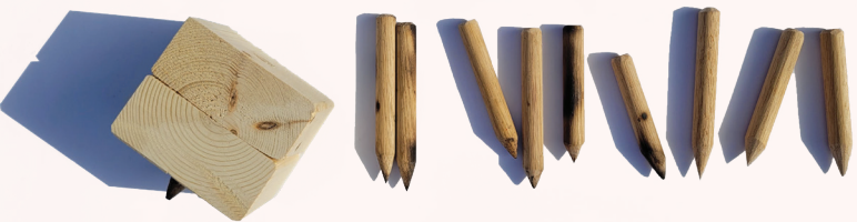
Fire-hardened tree nails. An assignment from early in the semester asked students to choose from a variety of all-wood fastener types and to create their own from scratch. Photo: Hanna Gross, Master of Architecture student.
