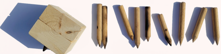
Fire-hardened tree nails. An assignment from early in the semester asked students to choose from a variety of all-wood fastener types and to create their own from scratch. Photo: Hanna Gross, Master of Architecture student.
