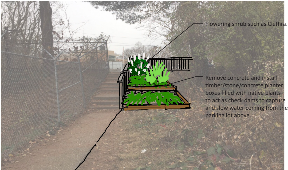
3 View of Terraced Conservation Landscape below Parking Lot
